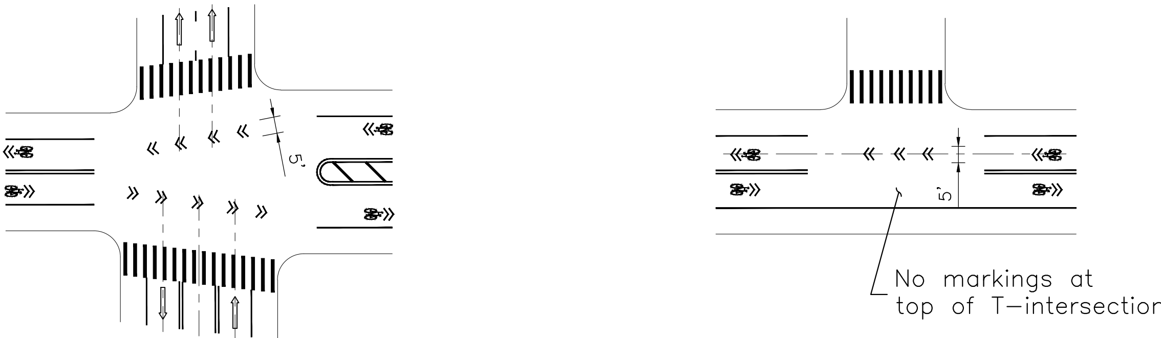
Detail D: Bike Route Intersection Markings
