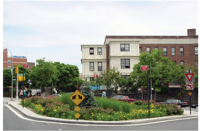
Planted triangle. Shorter plants are located near the edge to maintain sightlines: Macombs Road and Grand Avenue, Bronx (Credit: Parks)
