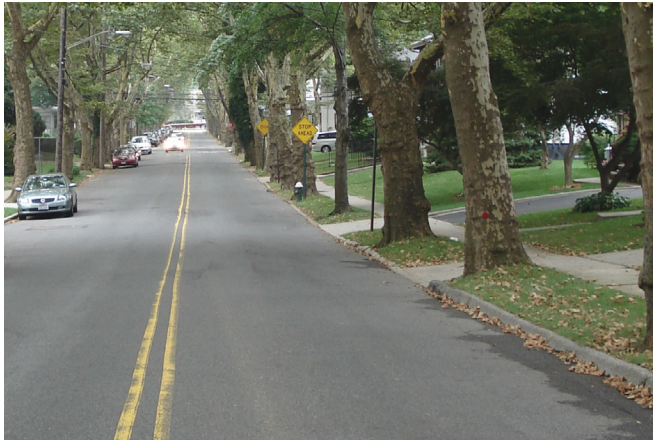
Ribbon sidewalk with turf grass and trees. Trees can be very large due to expanded rooting area afforded by adjacent lawns: Bancroft Avenue, Staten Island (Credit: Parks)
