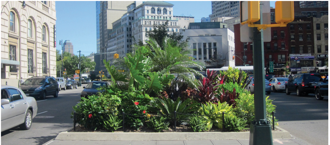
Planted median. Low plantings are located near the intersection to allow better visibility. Contrasting colors and texture add interest: Adams Street, Brooklyn (Credit: Parks)
