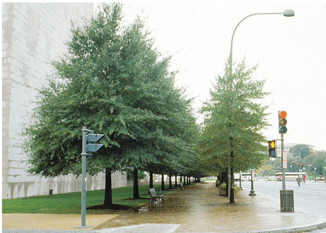
Willow Oaks planted at the same time with different available soil volumes. Note that the trees on the left, which have more soil than the trees on the right, are much larger. Pennsylvania Avenue, Washington, DC (Credit: Urban Horticulture Institute, Cornell University)
