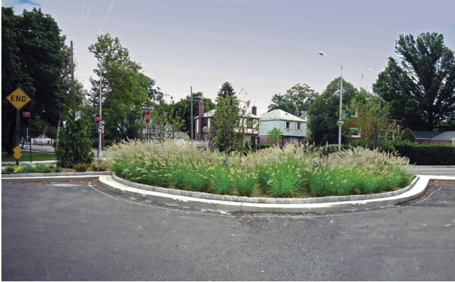
Planted area in a street end. These hardy grasses are appropriate for the context; they can tolerate salt and a wide range of soil conditions and provide year-round interest: 73rd Avenue, Queens
